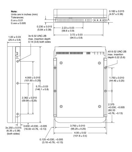
Figure 3. Mounting dimensions for the ST33240A and ST32531A—top, side and end view
