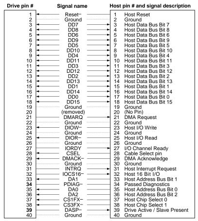
Pins 28, 34 and 39 are used for master-slave communication (details shown below).
